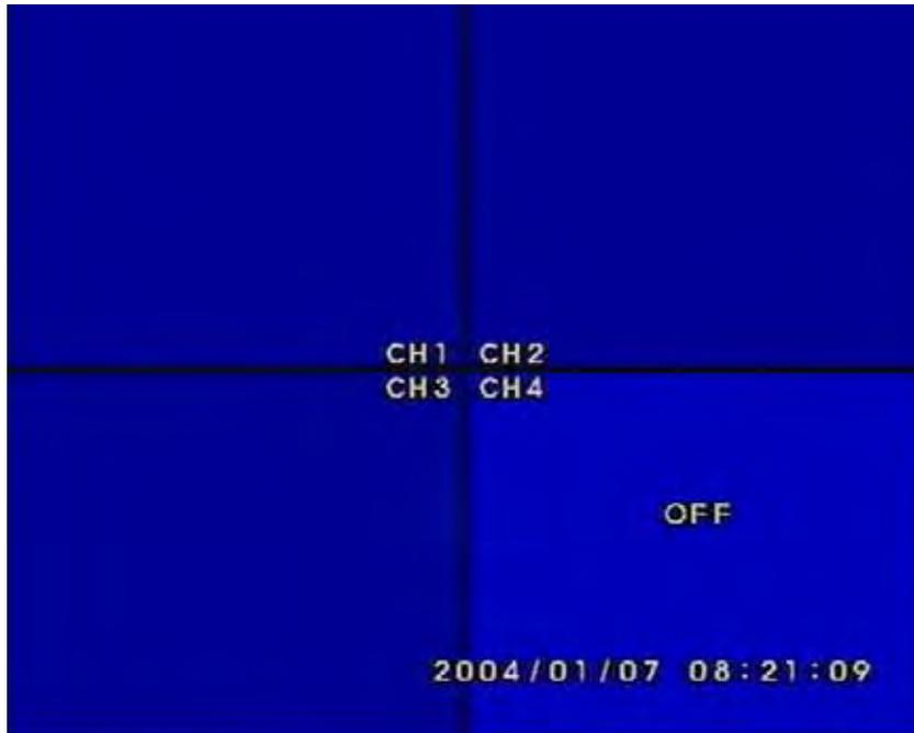
CH1-CH4 are the names of four channels. "OFF" means the fourth channel is set disabled.
