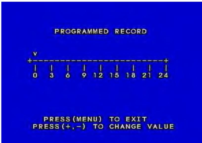
0-24 instead of 24 hours of a day, each hour can be setup to one of three states: T (time), S (sensor), - (normal).
