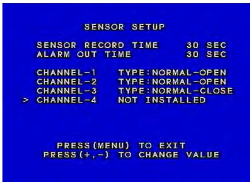
**SENSOR RECORD TIME:** The number indicates how long sensor recording will last after the sensor indicates the movements in front of the camera.
