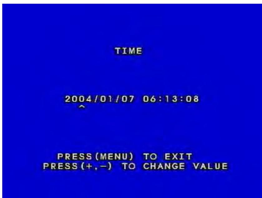
Push leftward button or rightward button to move the cursor, push add or decrease button to change the value.
